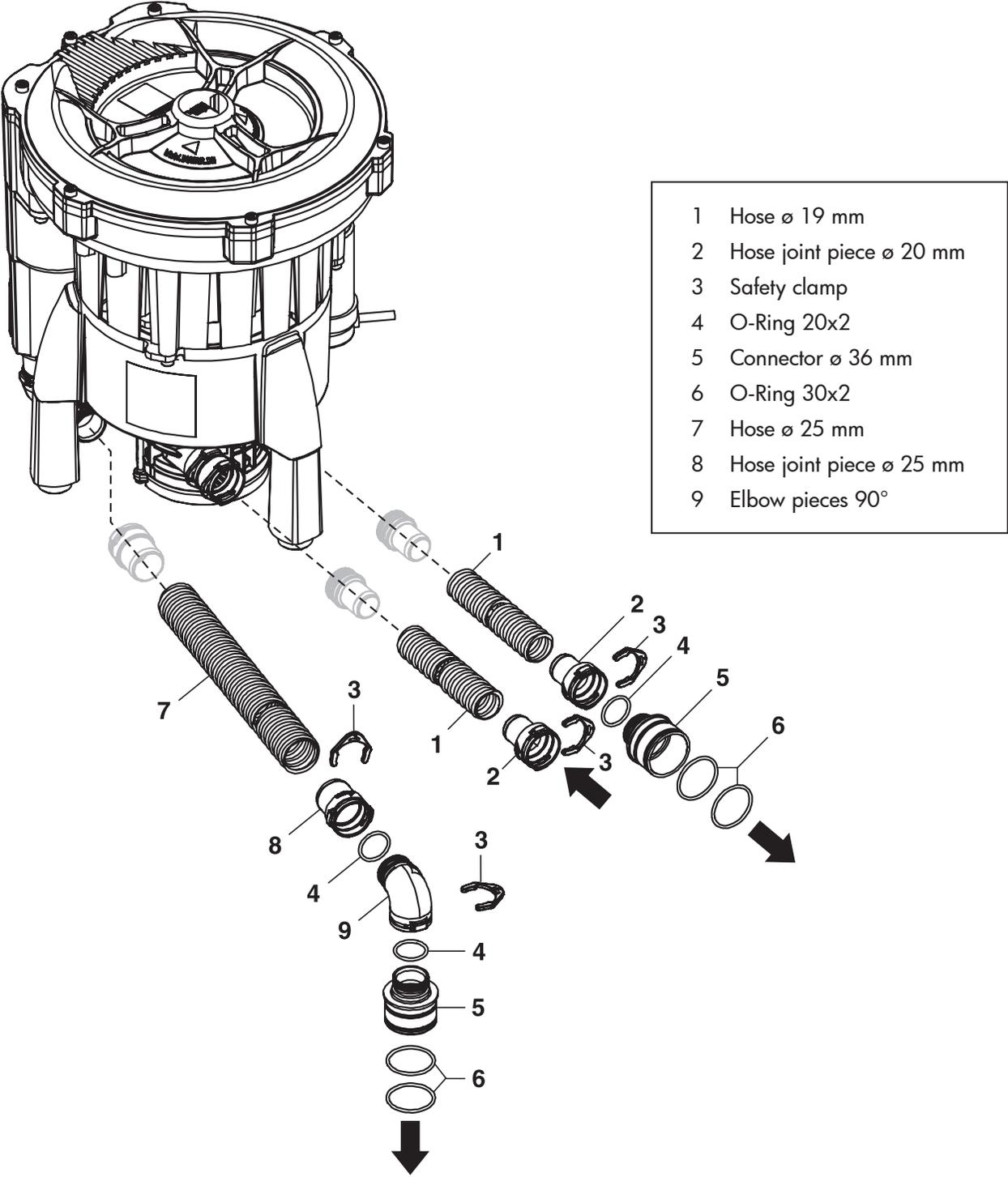
Figure 6. VIPER100 Parts Location Exploded View
