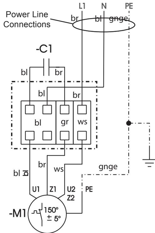
Figure 7. Motor Terminal Box Circuit Diagram
